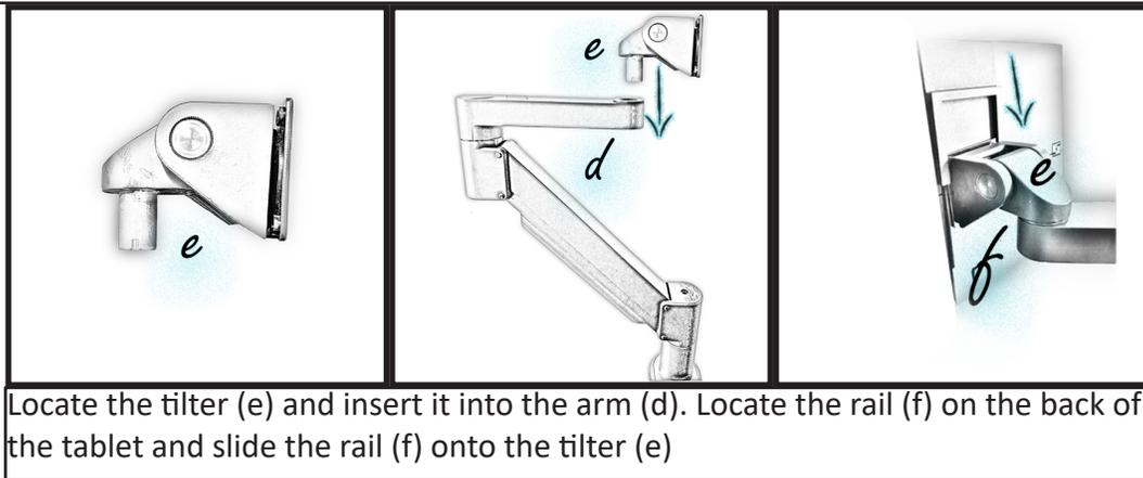
Locate the tilter (e) and insert it into the arm (d). Locate the rail (f) on the back of the tablet and slide the rail (f) onto the tilter (e)
