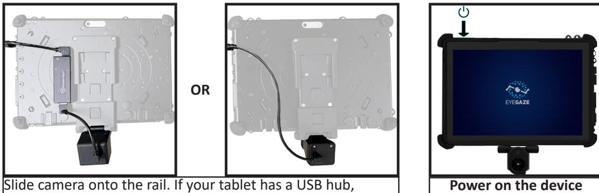
Slide camera onto the rail. If your tablet has a USB hub, connect the tablet to the hub, then the hub to the camera. If there isn't a hub, connect the tablet directly to the camera.
